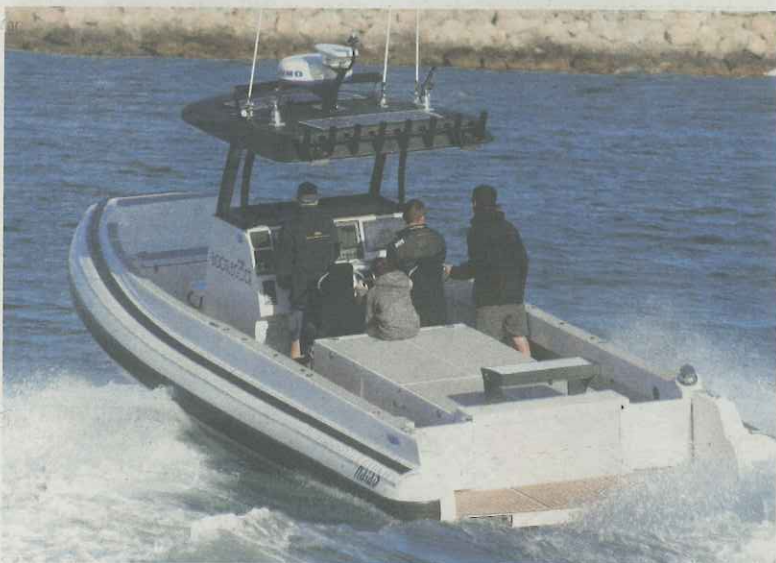
The engine box is high and it's easy to expose the mechanicals for any work.
